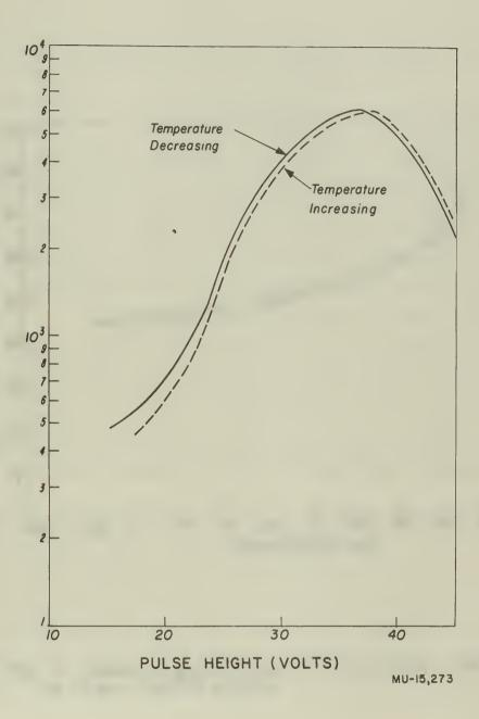
Fig. 8. Comparison of pulse height spectra in argon at 75 psi.
